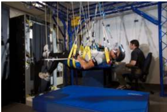
To mimic exercise done in a microgravity environment, test subjects run on the sZLS vertical treadmill.
